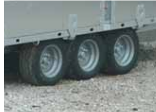
Tri-axle 3,500kg Max gross capacity 10" low rider wheels
