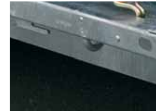
Rope hooks Multiple attachment hooks for securing loads with ropes
