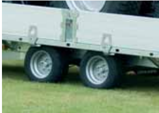
Twin-axle 3,000kg Max gross capacity 10" low rider wheels
