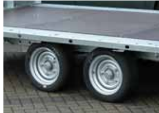
Twin-axle 3,500kg Max gross capacity 13" wheels
