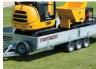
Aluminium sides Aluminium sides, steel headboard
