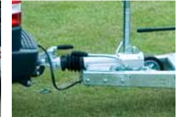
Towing height Tow coupling can be specified at 3 towing heights
