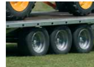
Suspension Rubber-in-compression suspension offers superior ride characteristics and long-term durability
