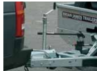
Jockey wheel Heavy duty, fitted as standard
